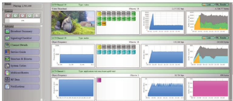
The StreamScope XM MT provides color-coded QoS indicators for multiple ATSC 3.0 channels.
