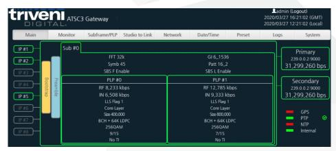
The Broadcast Gateway inputs ROUTE streams and outputs STLTP streams to ATSC 3.0 exciters.
